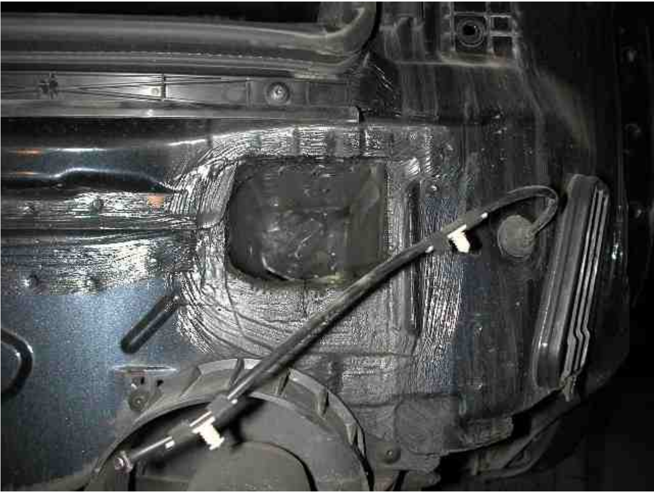
Being an '03, audi finally had the holes aligned, and no drilling was required. the hitch merely bolted right in.
