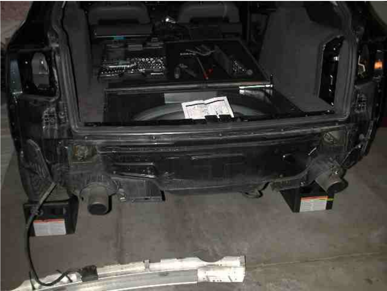
this next picture is looking into a hole where the bumper used to be held. the hitch slides into this hole, and the bumper mounts directly to the hitch.
