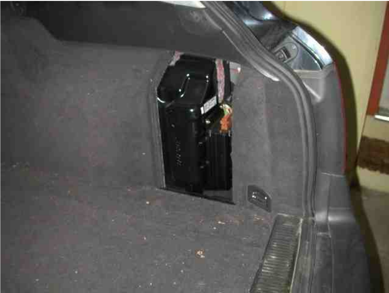
Quite a bit of the trim had to be removed, including the aluminum trim strip under the liftgate, the tie down latches and the cargo cover latch. Additionally, after removing the toolbox in the left rear, the bracket that holds it had to be removed:
